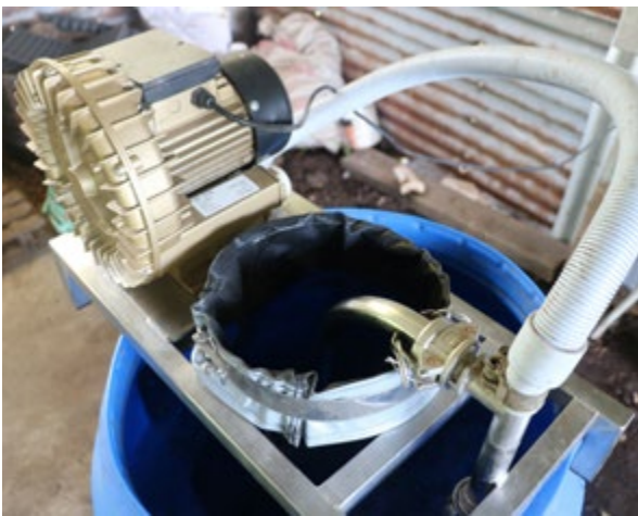
Aerator at Tutu releases oxygen into a nutrient-rich substance to produce compost tea.
